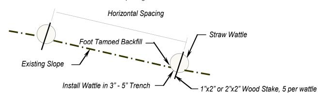
FIGURE 1 - Typical straw wattle installation
