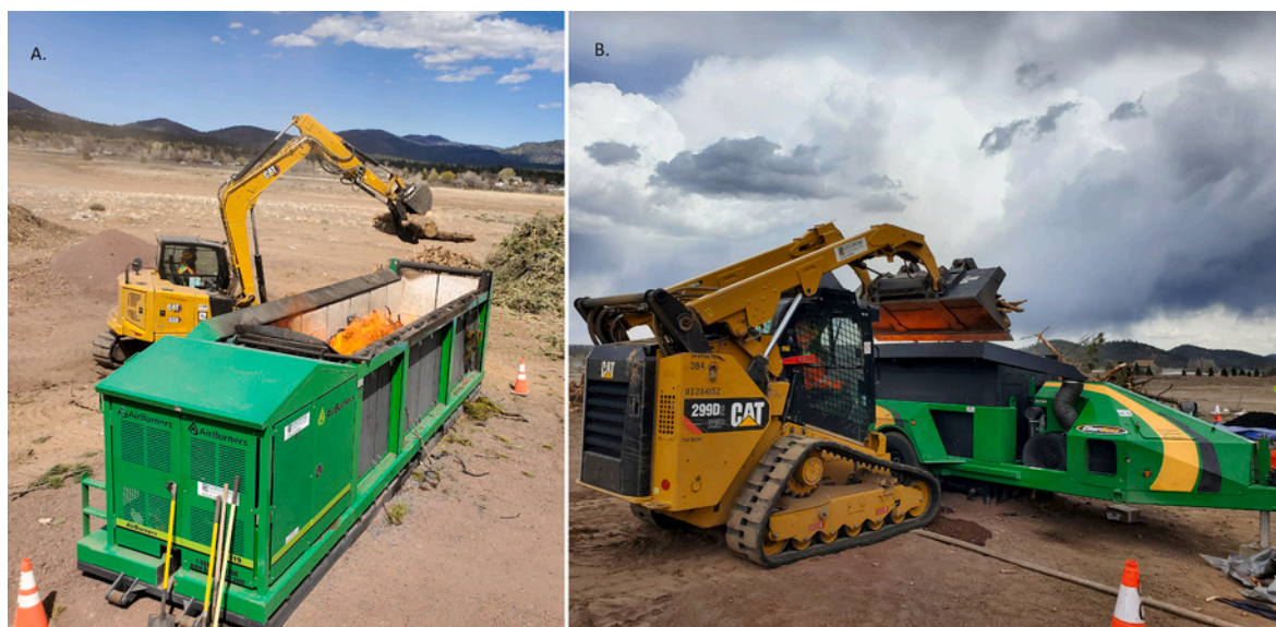
Fig. 5. (A) Loading FB with CAT 308 tracked loader and (B) Loading CB with CAT299D2 skid-steer tracked loader. The four-day burning schedule was based on hourly burning throughput for FB and CB machines, predicted wind speeds, and the quantity of biomass available for burning.
