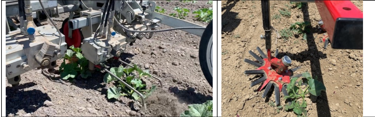
Figure 1. Robovator (left) and Steketee finger weeder (right) at WSREC and Dos Palos, CA, 2022.
