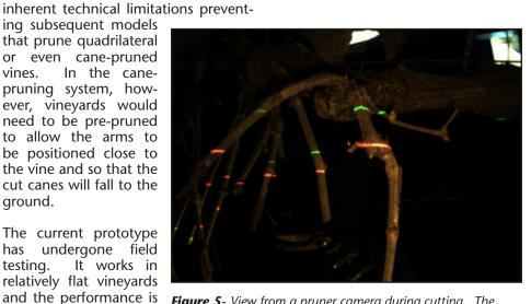
*Figure 5*- *View from a pruner camera during cutting. The* image is "upside down" as this orientation often affords better cutting positions. Red and green lasers are used to help quide the pruner to the cut point.
