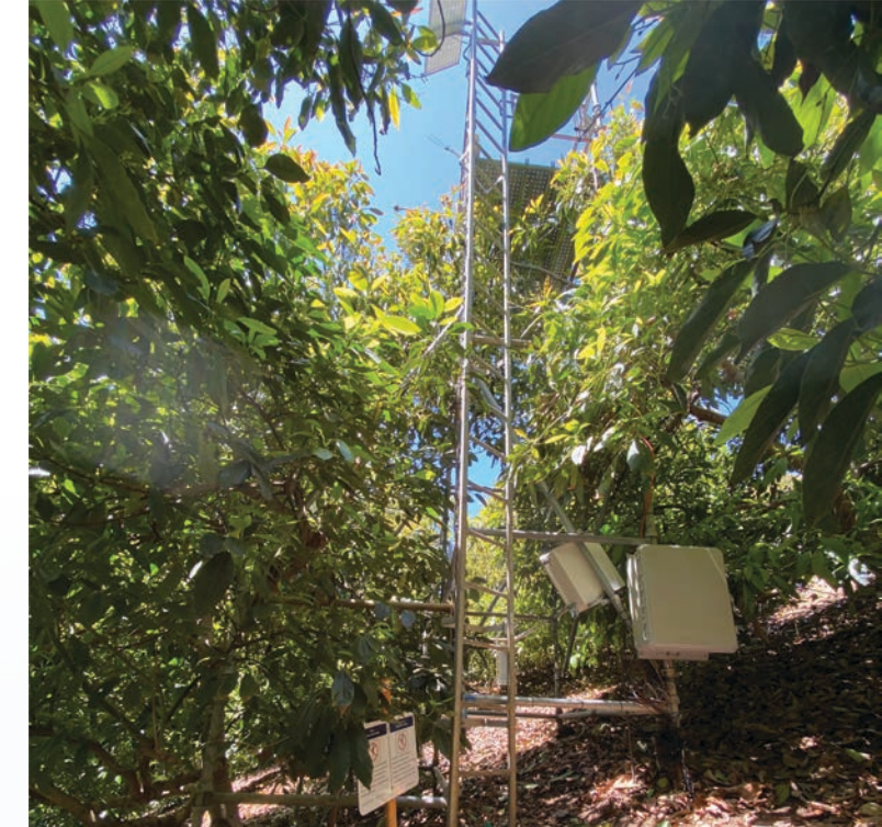
Fig 4. Ground view of surface renewal and eddy covariance ET station at the avocado site in Escondido.
