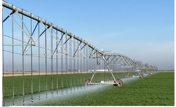
Fig. 14. An alfalfa field under linear move sprinkler irrigation systems in the low desert of California.
