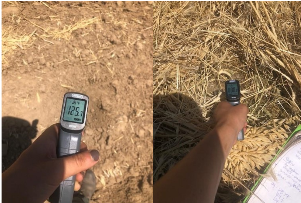
Soil temperatures on a disked cover crop section (left) and a mowed section (right)
