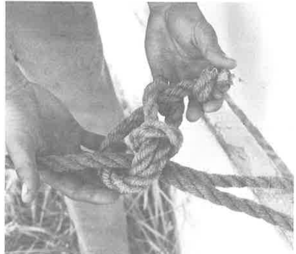
Step 4. Put the free end of the rope through the second loop
