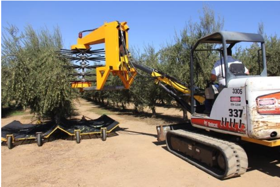
Fig. 2. A canopy contact harvester adapted from a jatropha harvester. Canopy contact harvesters have higher potential efficiencies with hedgerow orchards that can present a hedgerowed vertical fruiting wall to the harvester head. These orchards can be developed from existing orchards at, 96 -139 tree per acre, with mechanical pruning or developed as a hedgerow at higher densities, 202 trees per acre.
