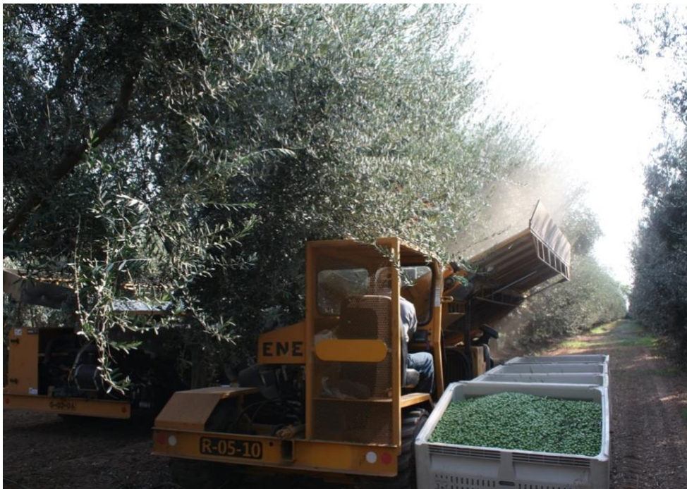
Fig. 3. Double sided trunk shaking pistachio harvester that can be used in existing orchards, 96 - 139 tree per acre, modified with mechanical pruning or hedgerow orchards at higher densities, 180-202 trees per acre.
