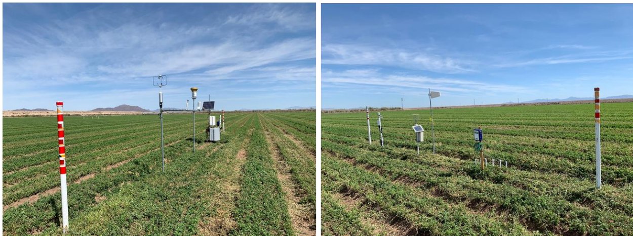
Fig. 1. A fully automated surface renewal and eddy covariance evapotranspiration tower at site B (left) and a multi depths soil moisture sensor monitoring station equipped along with Tule and NDVI sensors at site A (right).
