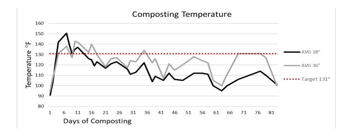
Temperature readings are taken at 18 and 36 inches depth and moisture and pH are also taken. A temperature of 131 degrees Fahrenheit for 72 hours is required to kill potential pathogens in the compost pile. On day three, the pile achieved the target temperature and continued through day eight. Water is applied as needed and extra wood chips and straw are available as the pile shifts and needs extra material.
