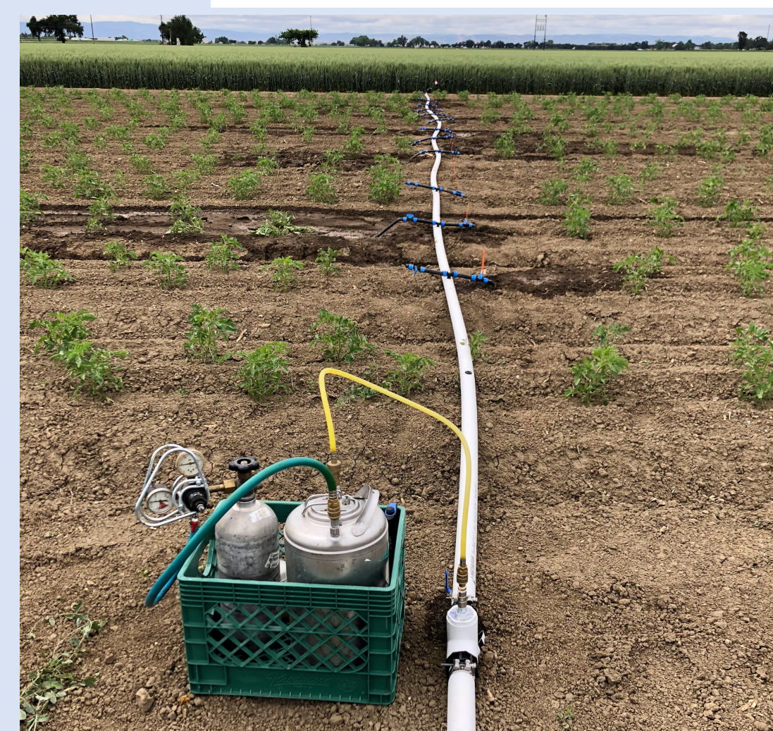
Figure 2. CO 2 injection system in efficacy study. The same system was used in the 2020 crop safety study.
