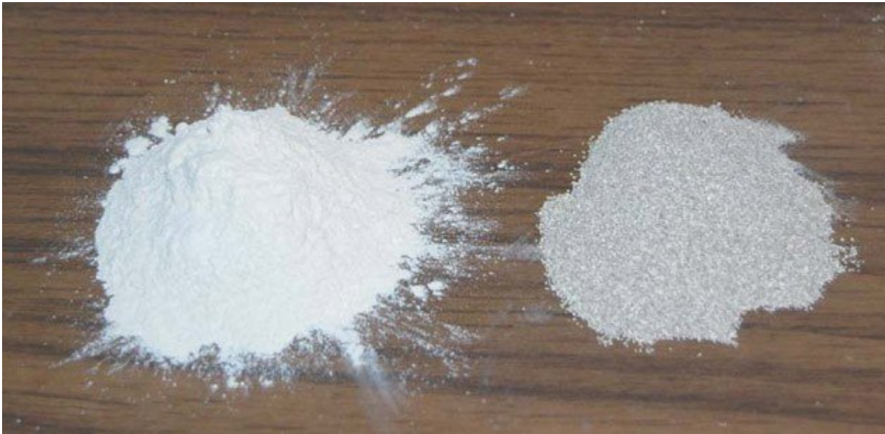
Figure 4: Two different types of bleaching clay. Shown on the left is a sample that is mixed with the oil, heated, and put through a filter press. On the right is a sample that is used as a filter in itself, which the oil is passed through. In both cases, the unwanted components in the oil are bonded with the clay, removing them.
