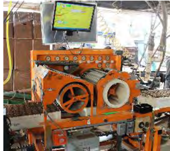
Figure 6.6 High-speed vacuum seeder sowing styroblocks in a forest nursery. Above the seeder is a display with information about the seedlot that is used to guide the sowing process.
