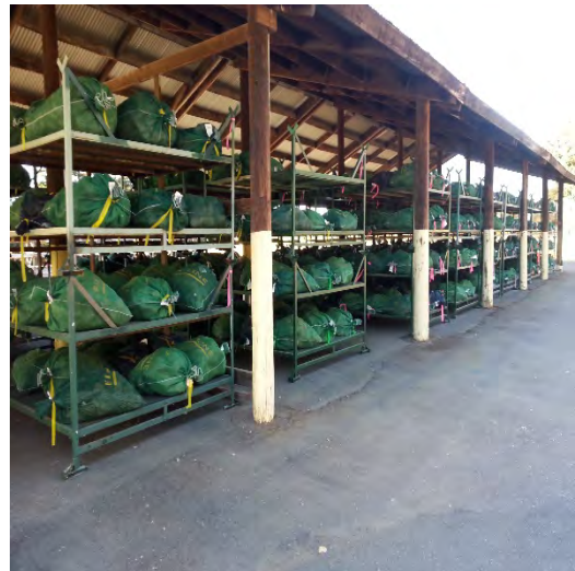
Figure 5.38 Cones air drying on racks in a cone shed.
