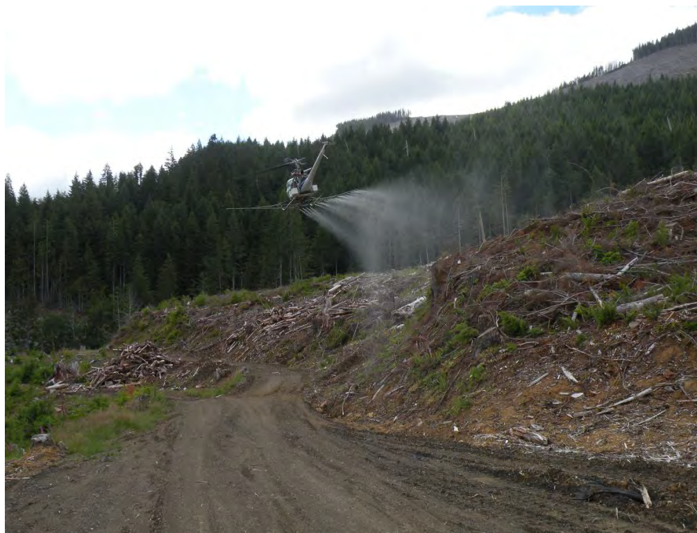
Figure 8.2 Example of a split boom application. Photo courtesy of John Mateski, Western Helicopter.
