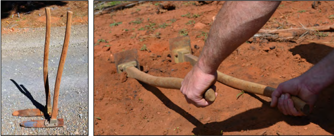
Figure 9.7 When planting flat or relatively gentle slopes, the 100-degree angled bracket hoedad (foreground picture on left) facilitates setting the blade into the ground at a right angle easier as shown by the hoedad in the left hand vs. the hoedad with a 90-degree angle bracket causing the planter's right hand to contact the ground when setting the blade at a right angle.
