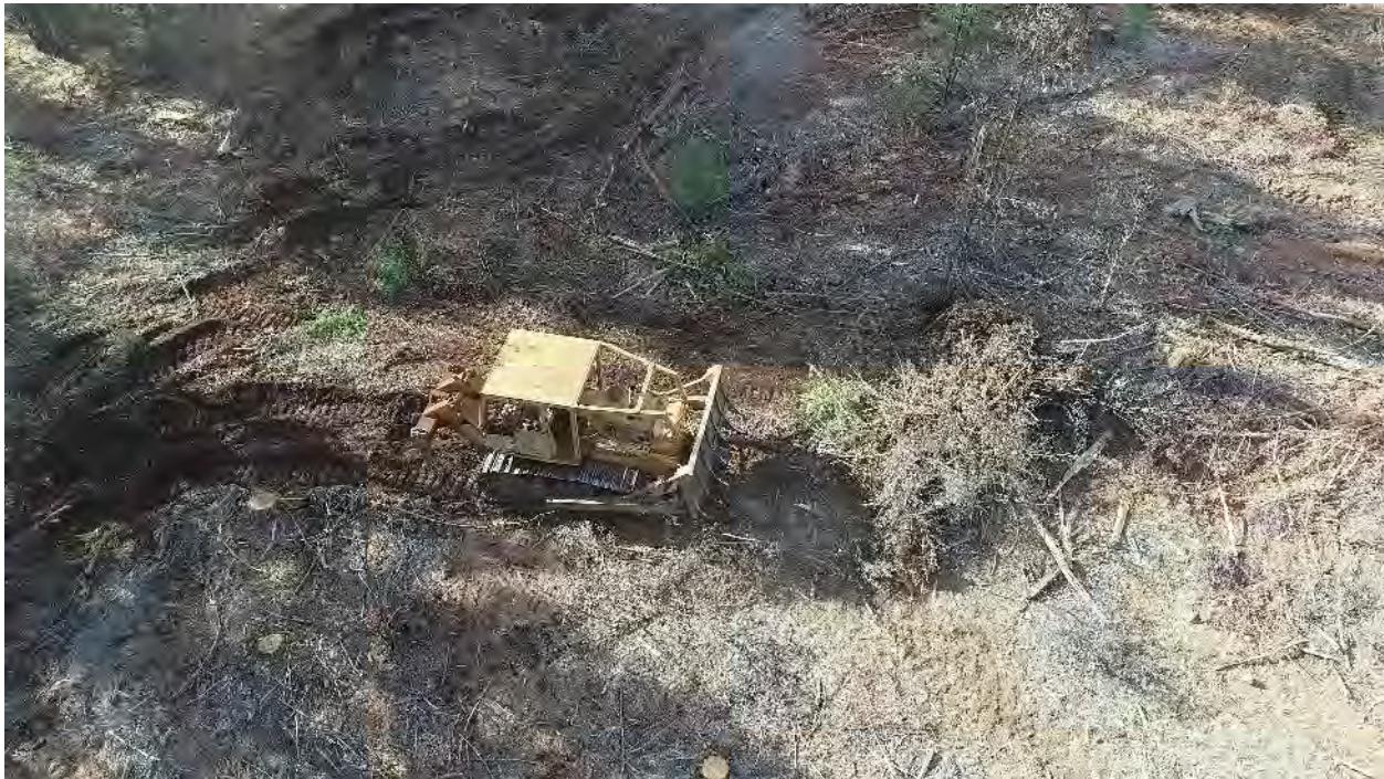
Figure 7.3 Cat with brush rake piling logging slash.
