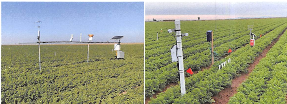
Figure 2. Fully automated ET tower (left) and a multi depths soil moisture sensor monitoring station equipped along with Tule and NDVI sensors at one of the experimental fields in Westmorland.
