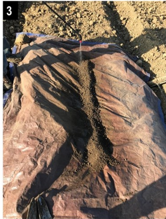
Picture 1-3: Soil samples were taken (1) followed by sieving (2) and moisture adjustment (3).
