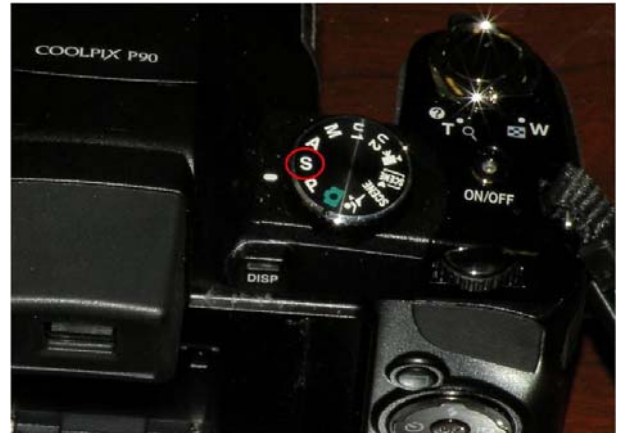
Figure 5 This dial shows the camera in a mode capable of adjusting the speed.
