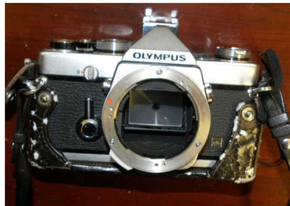
Figure 1. The inside of a film camera. The mirror and shutter behind it move when it shoots a photograph.
