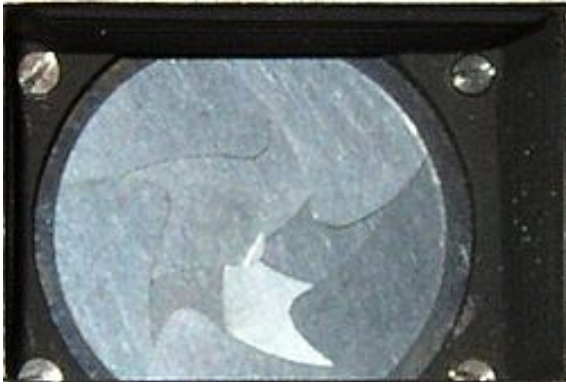
Figure 2. The circular diaphragm is a precision aligned plates that can open and close in a small fraction of a second.
