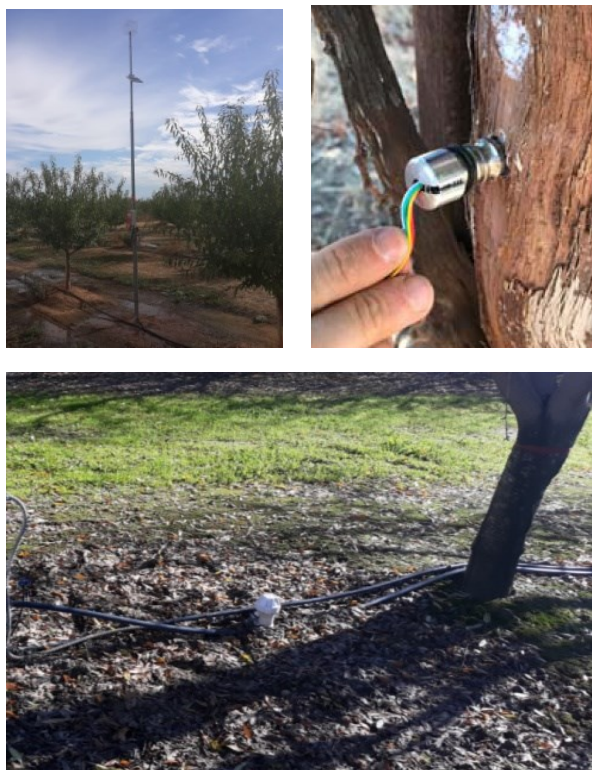
Figure 6. Irrigation scheduling technology. ET station (top left), plant water status sensor (top right), and soil moisture sensor (bottom).
