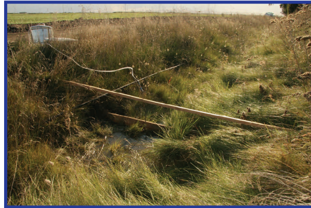
Automated sampling equipment is used for evaluating the effectiveness of vegetated waterways to reduce pesticide concentration in run-off.
