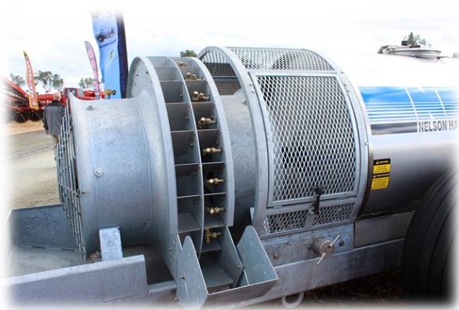
Photo: Conventional airblast sprayer with typical polar jet design. Credit: Peter Ako Larbi
