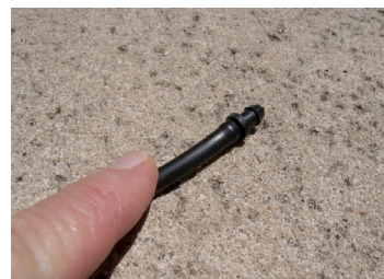
Goof plug inserted into open end of 1/4-inch tubing
