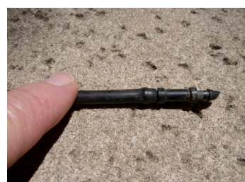
Coupler inserted in 1/4-inch tubing
