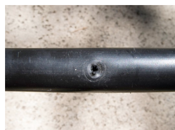
Hole punched in tubing
