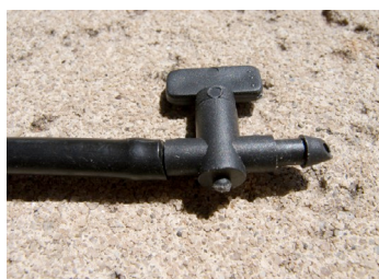
Valve connected to 1/4-inch tubing
