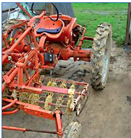
A basket weeder belly-mounted to an Allis Chalmers G at Pennypack Farm and Education Center in Horsham, Pennsylvania. The Allis Chalmers G was designed specifically for vegetable crop production, but is no longer manufactured. Photo: Andy Pressman, NCAT
