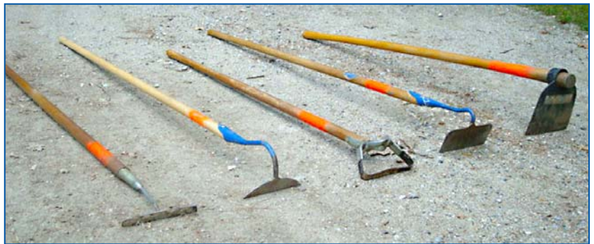
Hoeing works best on very small scales to remove young weed seedlings. There are several types of hand-held hoes. From left to right: a collinear hoe, a swan neck hoe, a stirrup hoe, a “regular” hoe, and an eye-hoe. Photo: Andy Pressman, NCAT
