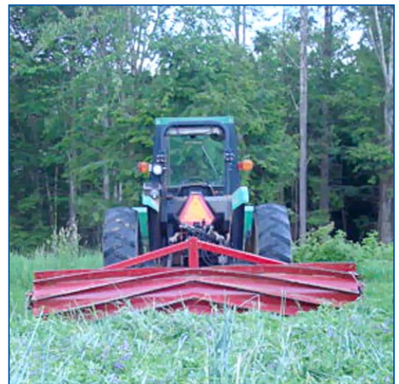
A roller-crimper mounted to a tractor. Roller-crimpers simultaneously kill the cover crop and create a thick layer of mulch into which seeds or transplants can be planted. Photo: Andy Pressman, NCAT
