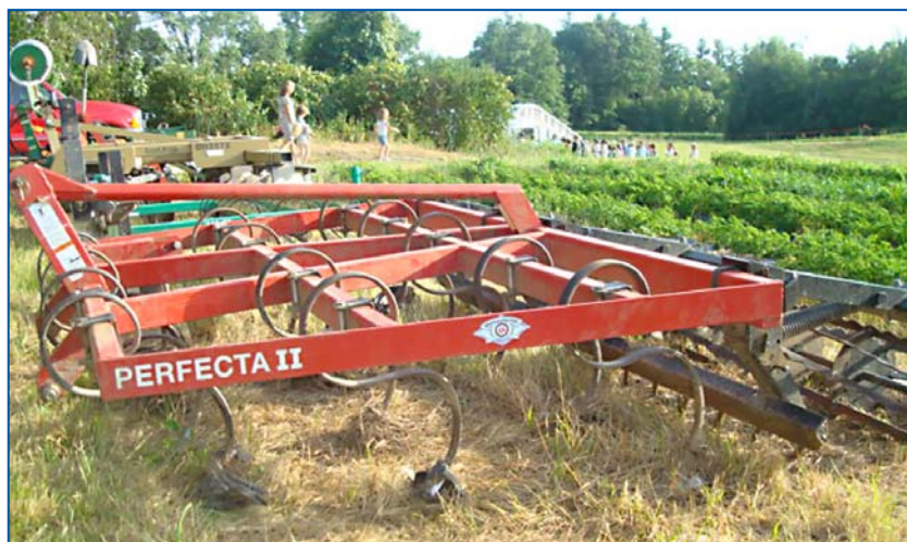
S-tine cultivator with sweeps, and a wheel that acts as a harrow on the back. Photo: Andy Pressman, NCAT
