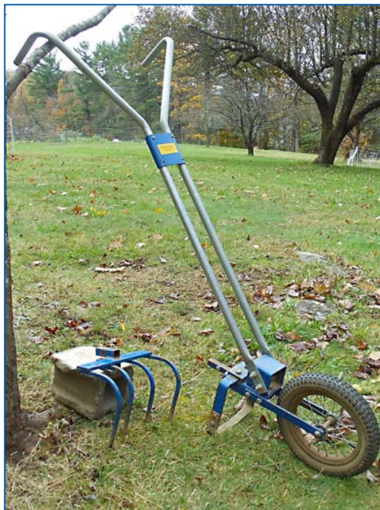
Wheeled hoes add an element of efficiency to the traditional hoe; smaller wheels are more efficient and easier to manage than larger ones. Here is a wheel hoe with a four-tine cultivator attachment. Photo: Andy Pressman, NCAT
