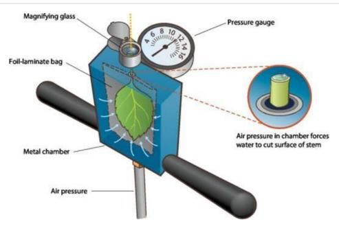
Figure 1. Schematic showing how water potential is measured in a severed leaf and stem (petiole) using a hand-held pump-up pressure chamber. Source: Adapted from Plant Moisture Stress (PMS) Instrument Company.
