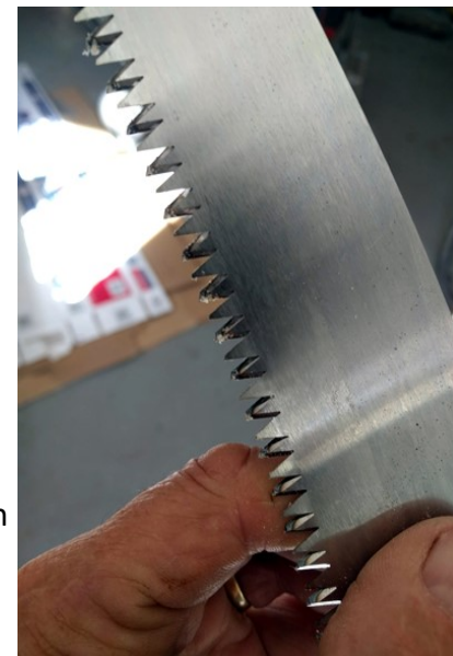
Illustration 1: Tri-edge saw blades are made from stainless steel and are not easily sharpened. When dull or bent they should be replaced.
