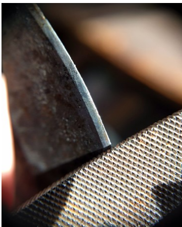
Illustration 2: To sharpen bypass clipper blades follow the angle of the bevel. Do not sharpen the flat side of the blade .
