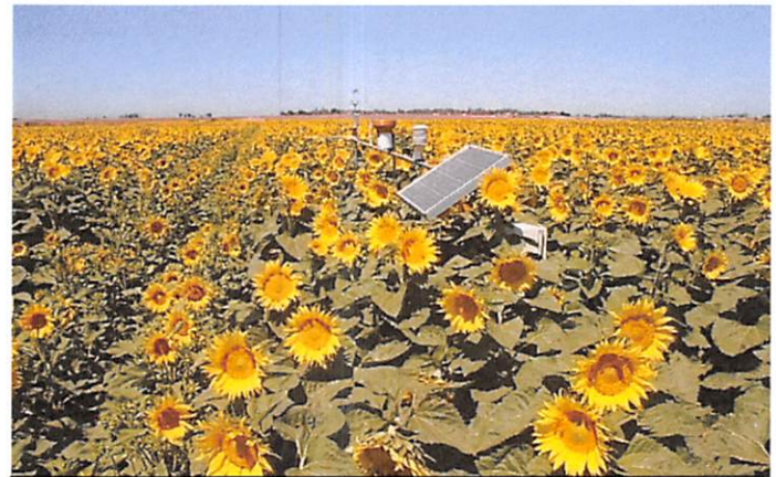
Fig. 2. Fully automated surface renewal and eddy covariance ET station at the experimental field.
