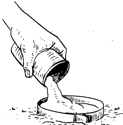
STEP 4. Pour plaster of Paris mixture over track.
