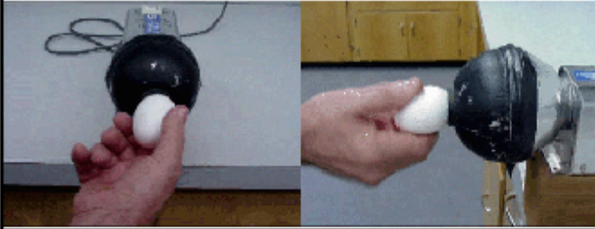
Figure 19. Official egg air cell gauge used in determination of the grade of an egg based on quality of interior contents.
