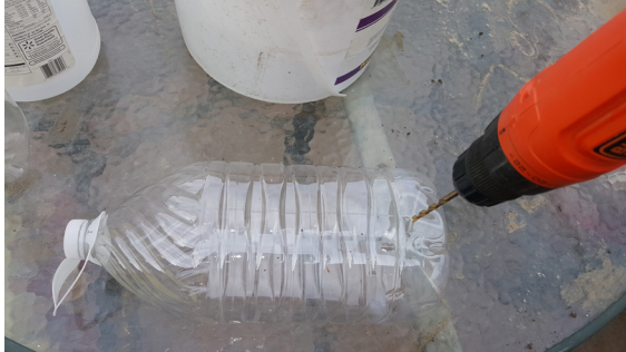
1. Drill drainage holes
