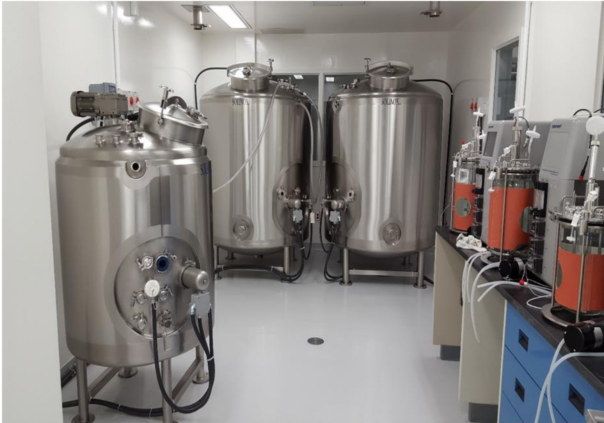
Secondary Fermenters in Background Primary Fermenter in Foreground
