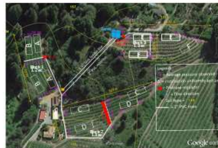
Figure 2. Map of the field with letters showing locations of DU measurements, and numbers showing pressure measurements in psi (in purple)
