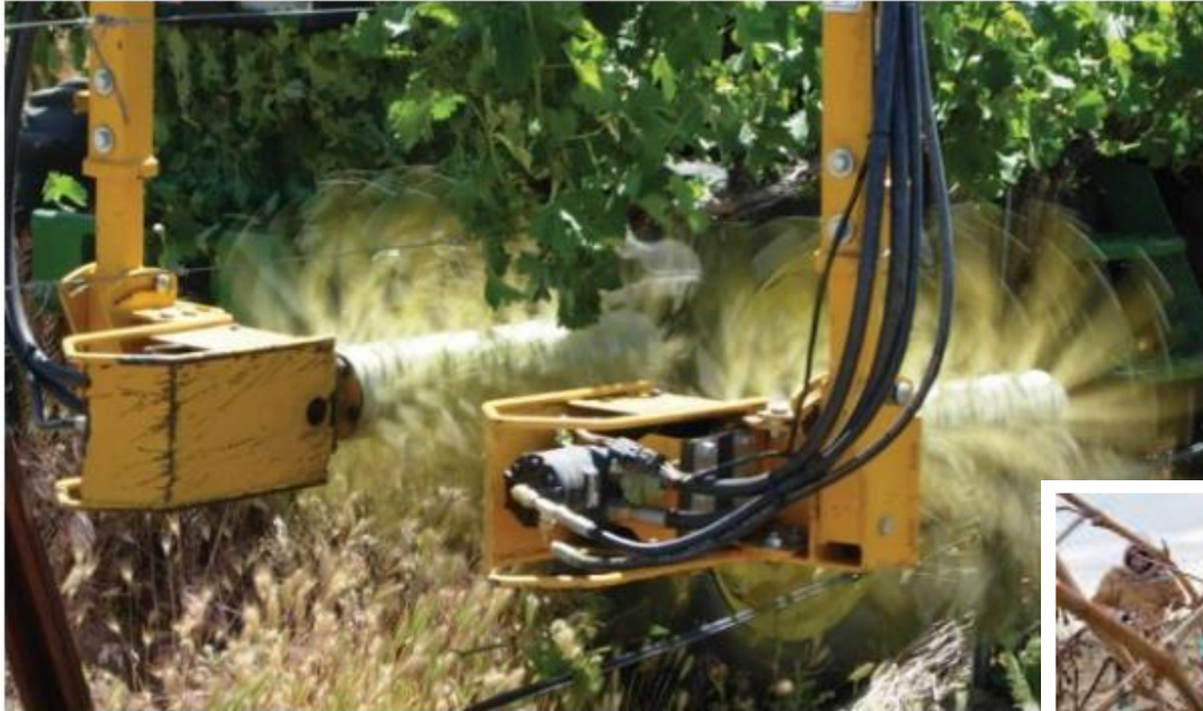
This trunk scrubber of the vMech system is used by Ste. Michelle Wine Estates to control trunk diseases. The device looks similar to a weed whacker with multiple strings.
