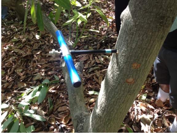
Fig.1 Wood core sampling from avocado using increment borer.
