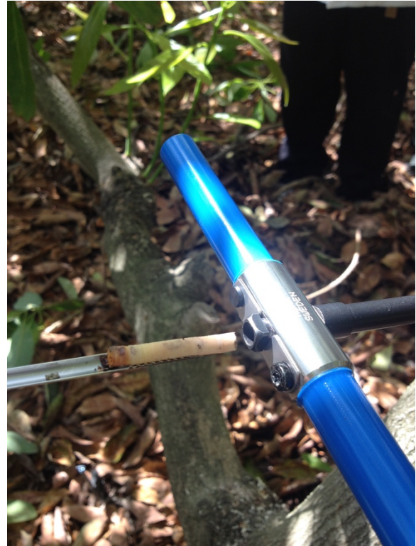
Fig.1 Wood core sampling from avocado using increment borer.
