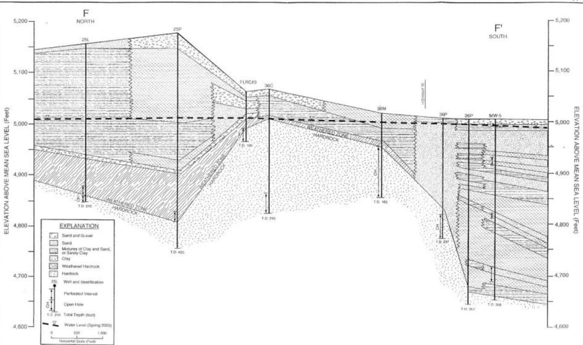
FIGURE 4 - SUBSURFACE GEOLOGIC CROSS SECTION F - F'
