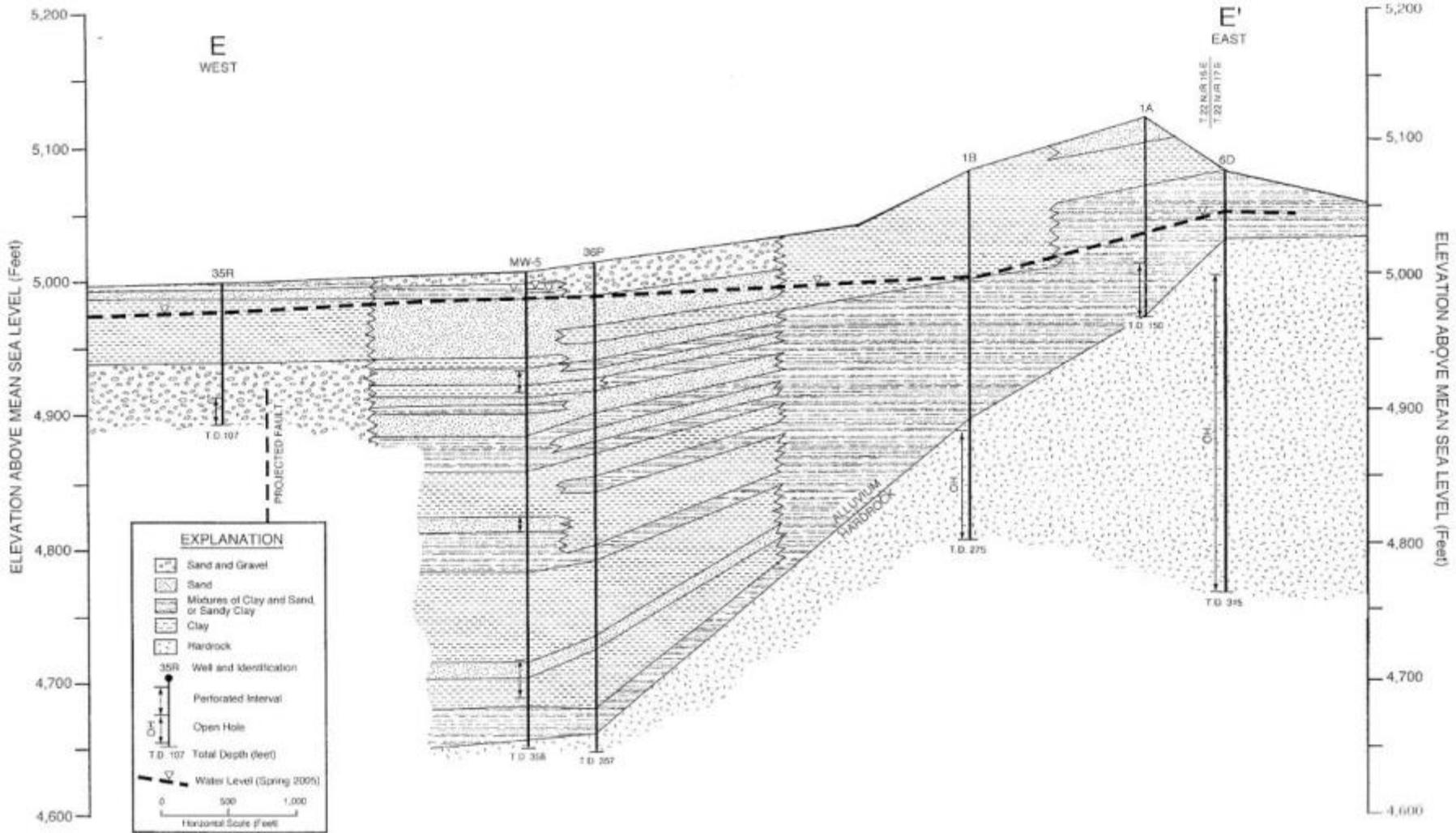
FIGURE 3 - SUBSURFACE GEOLOGIC CROSS SECTION E - E'
