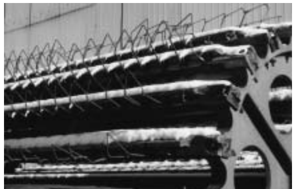
These retired hop rollers reveal the wire teeth used to strip the hops from the vines in mechanical picking.
