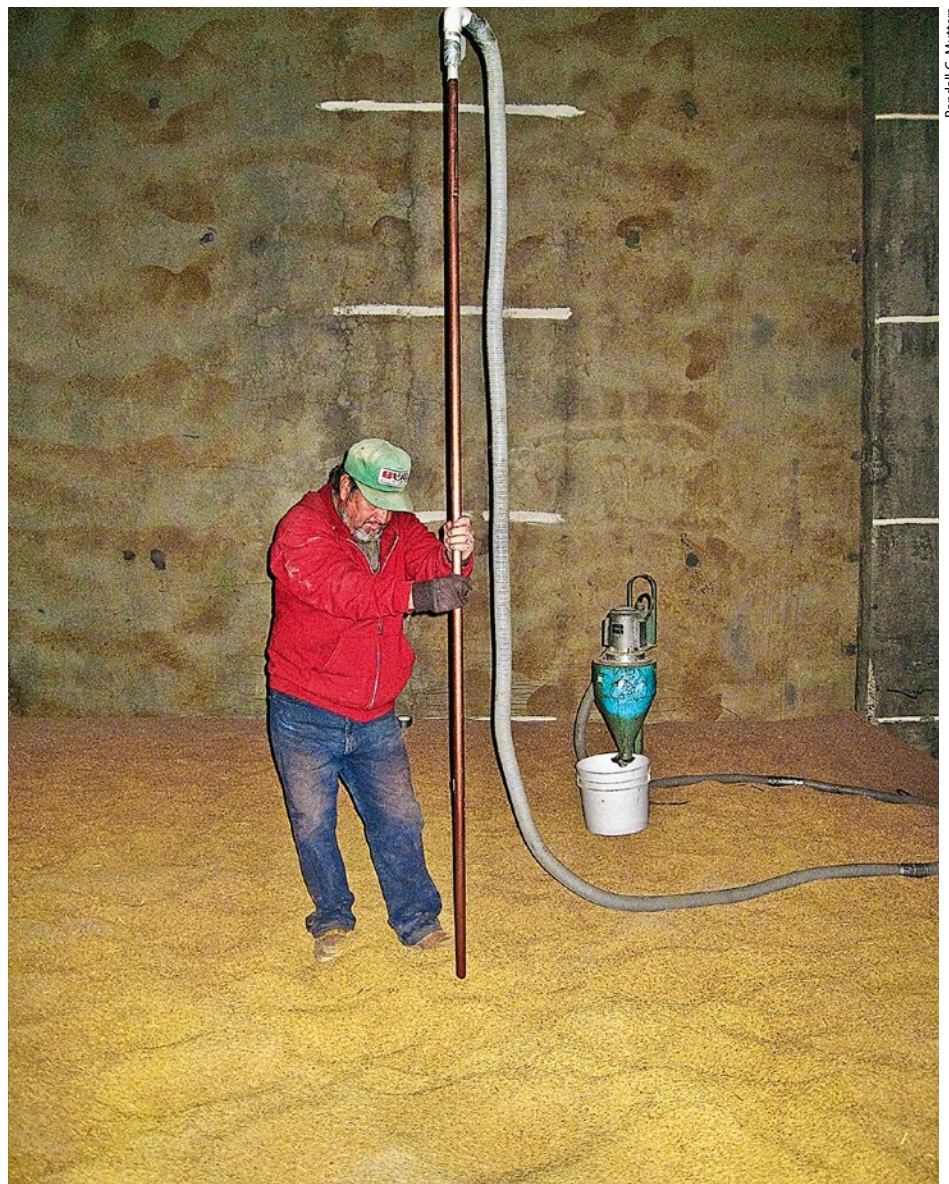
Stored rice should be inspected to determine its temperature, moisture content and sanitary condition throughout the storage period. In the authors' survey, almost all operations reported inspecting rice during storage. Above, a warehouse operator uses a grain probe to sample rice in a flat warehouse.
