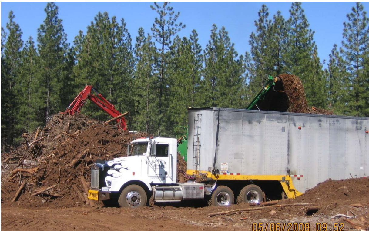
Chipping of biomass wastes from forest fuel treatments for use in SPI Lincoln energy recovery facility.
