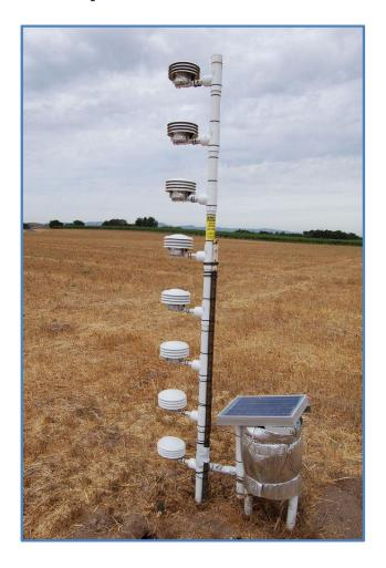
**Temperature Profile Tower:** Mark Battany, Viticulture and Soils Advisor, developed this instrument to measure air temperature at various heights to accurately quantify the potential risks and benefits associated with different vine training heights.
