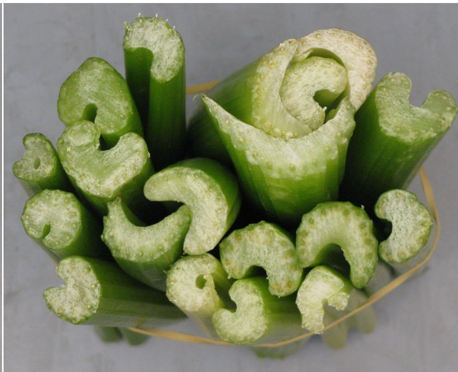
Waterjet cut (sharp nozzle)
