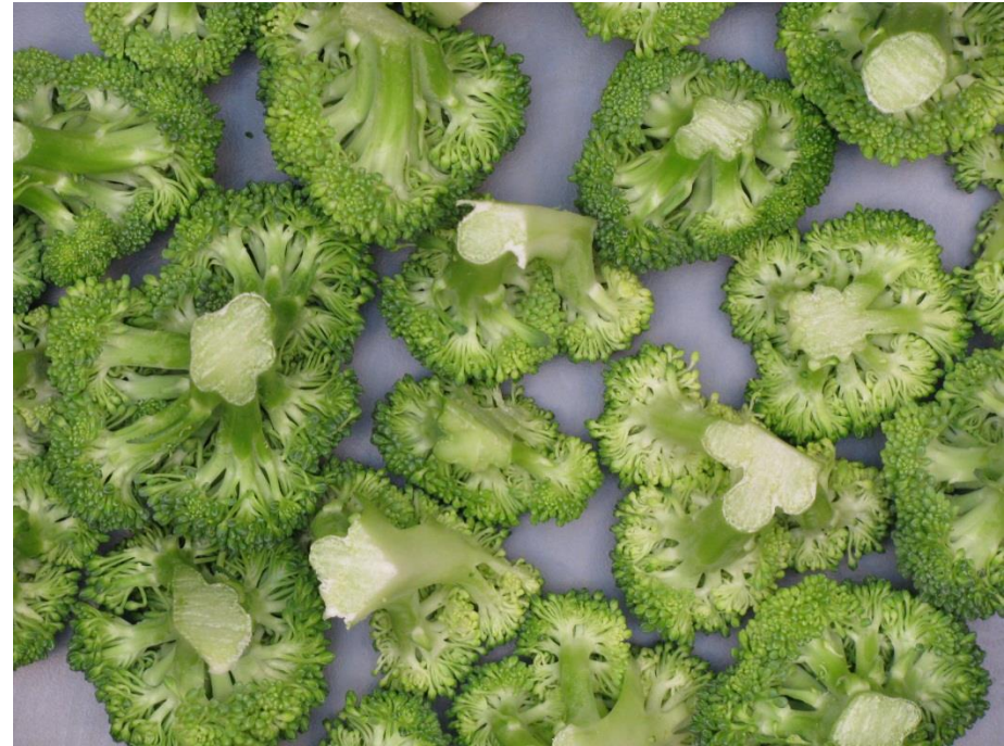
Waterjet cut (sharp nozzle)
