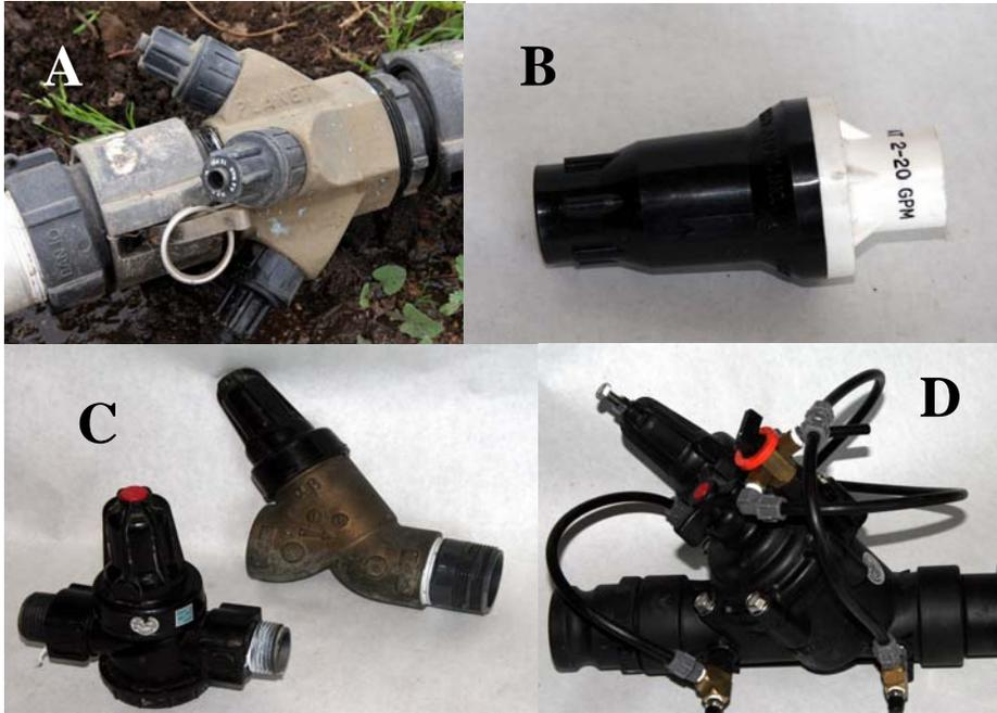
Figure 2. A brass pressure regulator preset for 12 psi can be used on 2 inch diameter pipe for flow rates up to 75 gpm (A), a plastic pressure regulator preset to 15 psi can be used on 1 inch diameter pipe and for flow rates from 2 to 20 gpm (B), adjustable plastic and brass pressure regulators for 1 inch and 1.5 inch diameter pipes, respectively (C), and a plastic pressure regulating valve with pilot for 2 inch diameter pipe (D).
