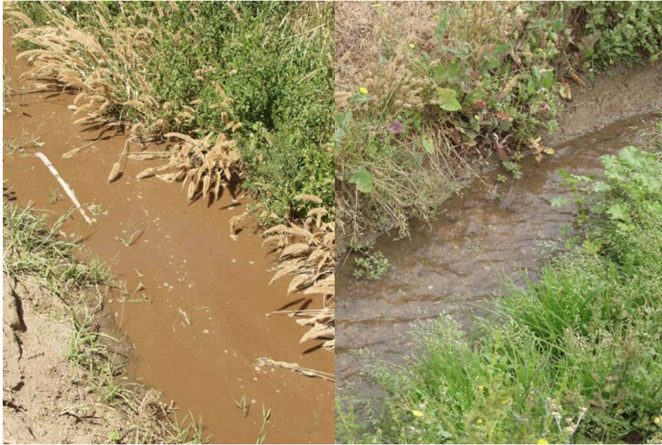
Figure 1. Run-off from overhead sprinkler water treated with 5 ppm PAM (right) and untreated (left).
