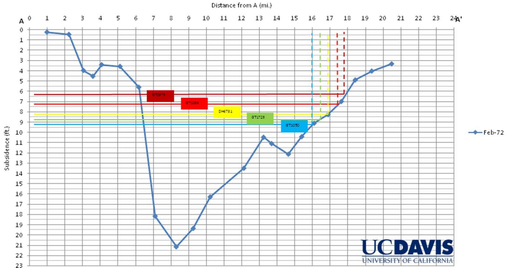
**Figure 56** Digitized 1972 subsidence profile (A-A') showing method for locating NASL benchmarks.
