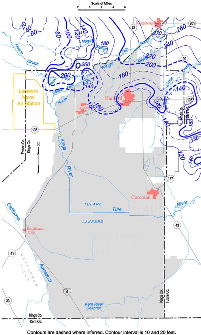
**E 46** Unconfined aquifer groundwater contour map, Tulare Lake groundwater basin, Spring 2005.
