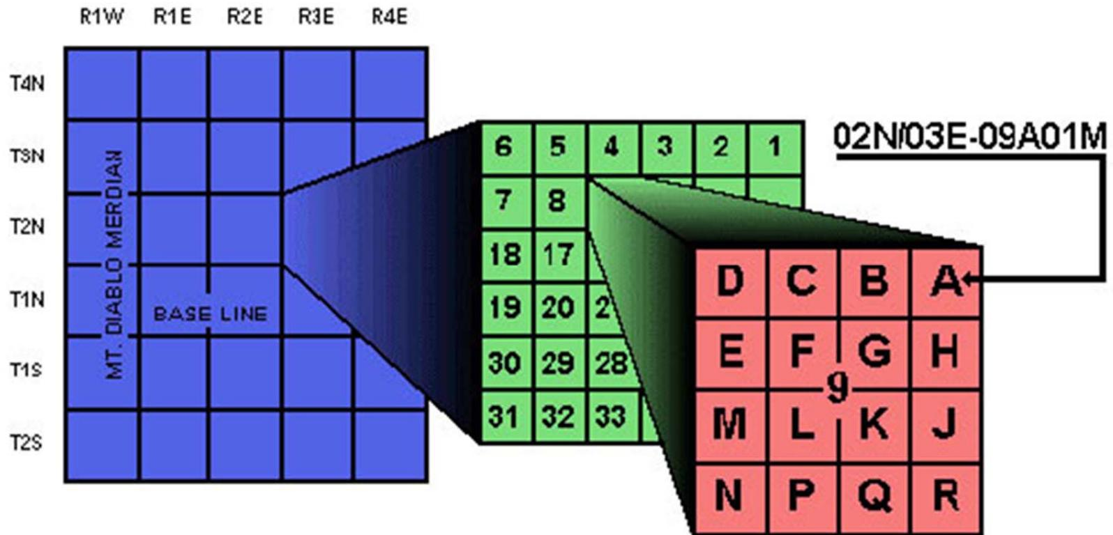
**Figure 1** CDWR well-numbering system (CDWR website, 2010).
