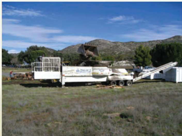
Commercial-sized tub grinders may be required to handle large pieces of oak.
