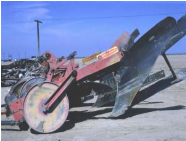
Plate 5. Moldboard plow capable of penetrating 3 to 4 feet.
