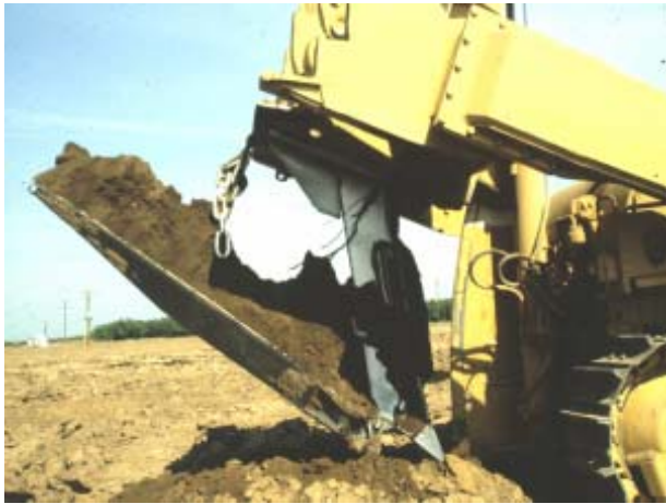
Plate 4. Slip plow with a following foot to further lift and mix layers.
