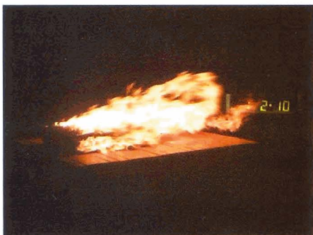
A 12" X 12", 3-layer sandwich, 'brand' used for the above-deck exposure tests. Each Douglas-fir stick is 3/4-inches square.
