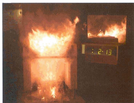
A burning plastic composite deck experiences accelerating combustion while at the same time dropping flaming debris. The mirror on the right shows a view from the top of the deck.
