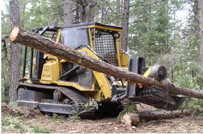
Figure 17. This small tree processor delimbs and cuts trees to the desired length.
