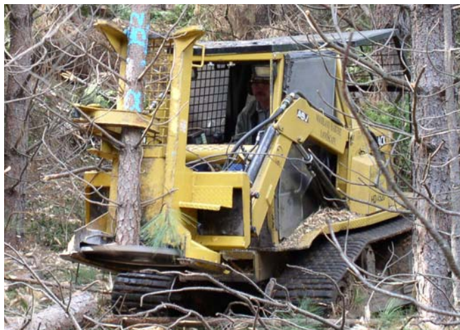
Figure 16. This feller buncher, mounted on a skid-steer, grasps a tree and cuts it using a circular saw blade.
