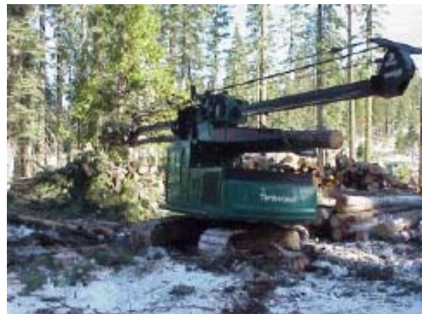
Figure 35. Log being processed by a stroke-delimber.
