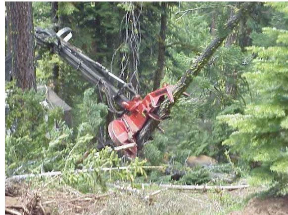
Figure 31. Feller buncher transporting the cut tree to a doodle pile.
