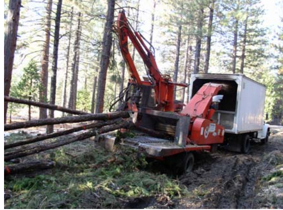
Figure 37. Chipper self feeding small logs and blowing chips into a chip truck.
