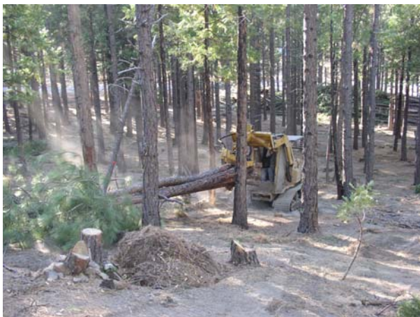
Figure 34. Doodles being transported to a landing by a tracked skid-steer with a log grapple attachment.
