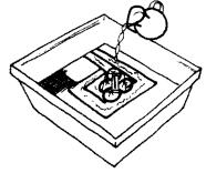
2 to 3 days before the hatch, stop turning the eggs, and fill both the 'THERMAL' and the 'CIRCULATED' troughs with water. **STEP 13**
