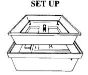
Unpack the incubator from box. Use thermostat bracket as handle to remove the incubator top from inside the bottom, where it is packed for shipping.
