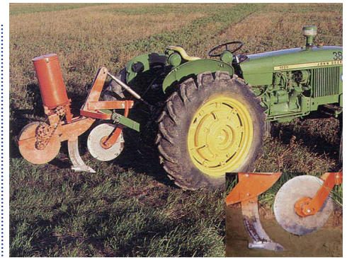
Figure 4. Mechanical bait applicator.
