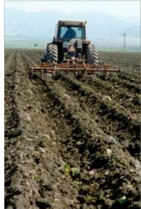
In a 3-year study, intermittent deep chiseling and ripping resulted in higher fresh lettuce yield and fewer symptoms of lettuce drop disease. A minimum-till ripper in the field undertakes the last step of the four-step deep minimum tillage program.
