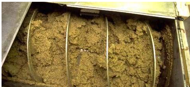
Thick, crumbly, dry paste from Frantoio variety olives that does not emulsify and separates easily. Note clean paddles due to coating of free oil
