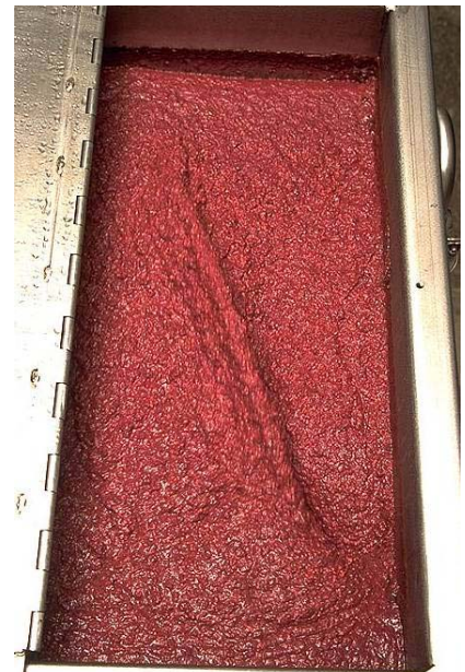
Wet, over-watered, very ripe Manzanillo paste that forms an emulsion between oil and water, which increases losses in the pomace or wastewater. Note paddles in the malaxator are covered with sticky paste.
