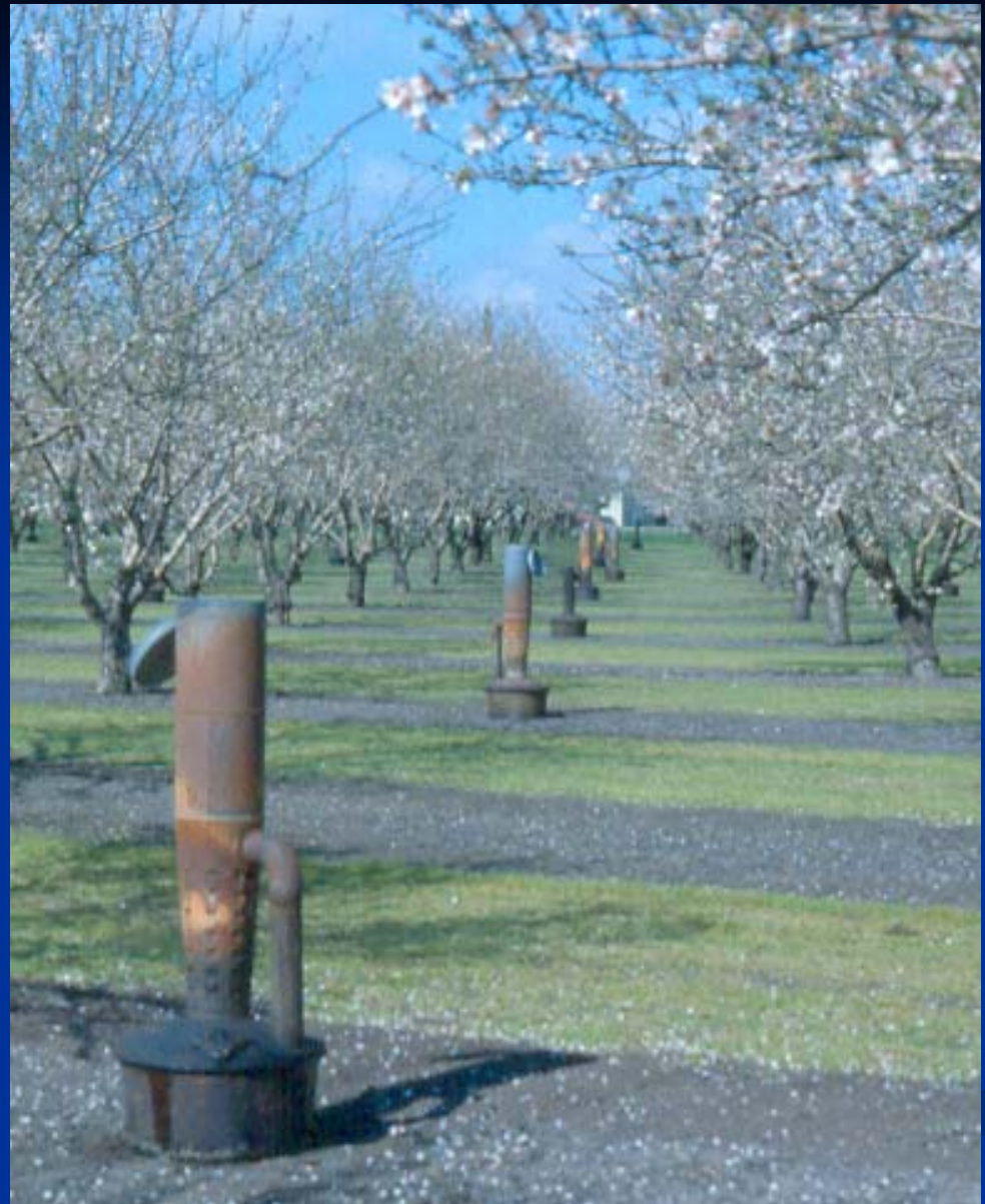
UC Return Stack Orchard Heater – developed by Ag Engineering at UC Davis
